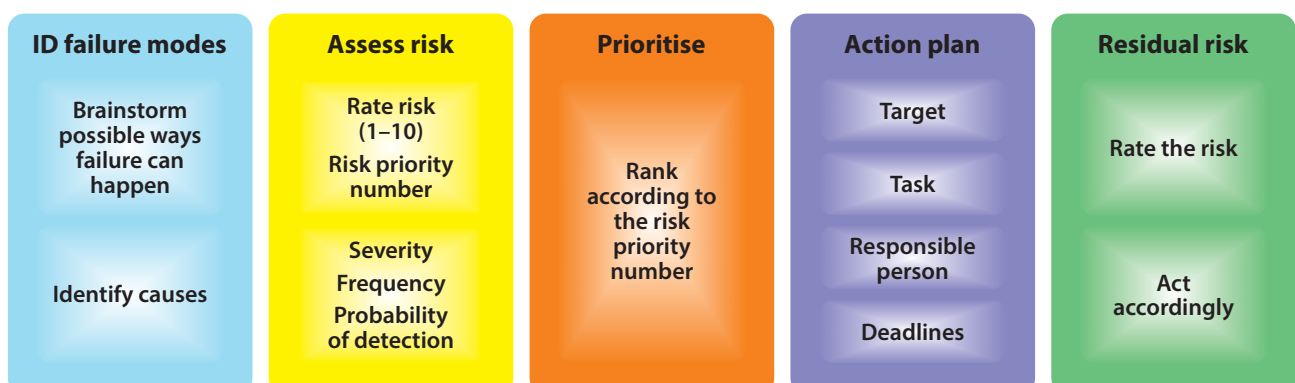
Figure 3.1. Failure mode, effects and criticality analysis (FMECA)
